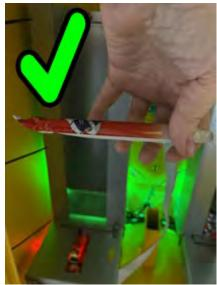
Seam in correct loading position
