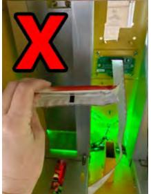
The seam is in the wrong loading position. Loading this way may cause the pack to get caught in the chute.
