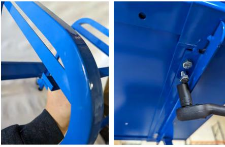
(NOTE: Slide the Flipper into place so the locking brackets fit between the legs)
