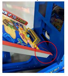
4. You can access the situation and see what is creating the jam. Free the jam and make sure the chute is clean and free of debris.
