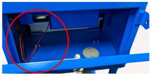
NOTE: When removing be careful of pulling on any cords that may be showing here. These are low voltage cables for the LED's
