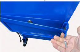
2. Open the bottom section on the back using a Set of #2 Keys
