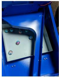
NOTE: The playfield's cord has enough slack so you can remove the playfield however if the slack is NOT pulled thru the back end the cord can create a jam of the capsules.
