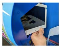
6. Slip the new monitor in the same way and now close it all up and plug in the monitor's power supply and USB Drive and we are good to go!
