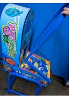
2. Now we can pull back on the trim leaving us enough room to remove the plexiglass. The plexiglass is one solid piece so lift it straight up to remove it safely
