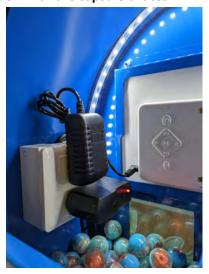
NOTE: There are two power supplies in the top section of the machine. One is for the monitor, and one is for the LED's. The machine doesn't require power to run just to power the video and LED's
