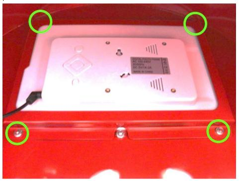
Once the entire plate pops out simply pop the monitor out and replace with the new monitor and once again tighten the 4 nuts.
