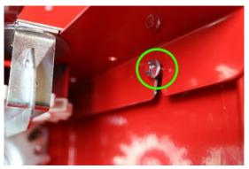
**Step 4:**Now you can remove the entire gear shelf out of the machine.
