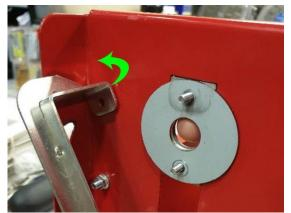
**SteP 3:**Remove both the circle plate and the square plate on the opposite side.
