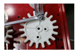
**SteP 7:**Replace with the new gear and reassemble
