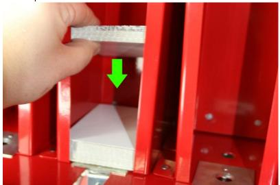
Note: Make sure the cardboard sleeve's perforated edge/ seam is facing the front of the machine. Otherwise the sleeve can get caught.
