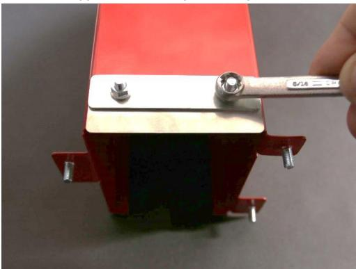
Note: I find the best way to find the height bar's "sweet spot" is to drop the bar as far as it can go then raise it halfway up and tighten.
