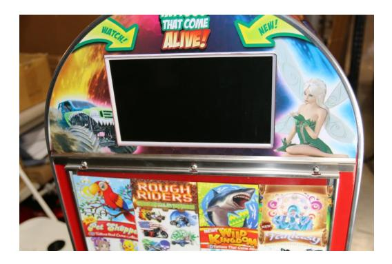
Now you can place the display bar back along the top of the plexiglass and reattach the 3 screws and nuts.
